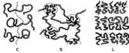
Fig. 8-16 Arrangement of A-blocks with A-units ● and B-blocks with B-units ○ in diblock copolymers A_n-B_m (C, L) and in triblock copolymers A_{m/2}-B_n-A_{m/2} (S) [8]. Note that m and n in this figure refer to the respective space requirements and not to the amounts of monomeric units. C: Compatibilizer at the phase boundary - - - between A-polymers and B-polymers. S: Spherical A-domains in a continuous B-matrix ( m \ll n ). L: Lamellae with A-layers and B-layers ( m = n ).
