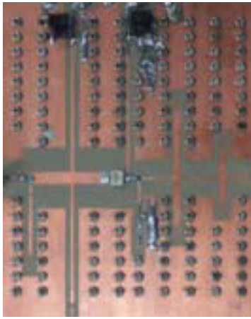
Figure 6 Photograph of the implemented amplifier using MRF282SR1. [Color figure can be viewed in the online issue, which is available at www.interscience.wiley.com ]
