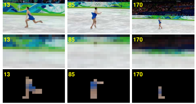
Figure 4. Sequential estimation of blockwise appearance models in the skating sequence. (Row 1) Input image. (Row 2) Mean colors of background block appearance models. (Row 3) Mean colors of foreground block appearance models.
